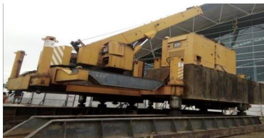
Gambar 2. 1 Alat *Hydraulic Static Pile Driver* (HSPD)
