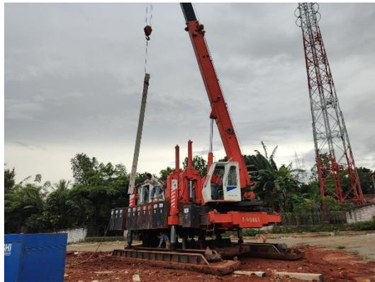
Gambar 4. 1 Alat Hydraulic static pile driver
